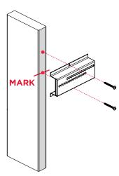
2 Mark holes through bracket mounting plate, drill 1/8" pilot holes and install screws into stud. Tighten screws firmly.
