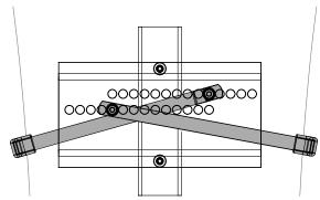
Insert bar with bent end into the left side and attach to the top row of holes with provided small screw.
