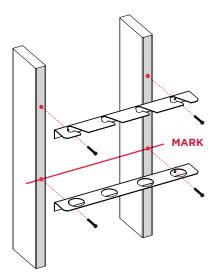
2 Both wood screws must be fastened into a stud inside the wall.
