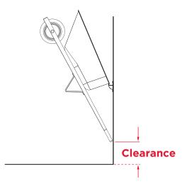
1 Verify the height of the hook is at a convenient location and that the wheelbarrow or ladder has adequate clearance once hanging.
