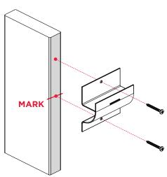
2 Position the bracket on the wall with enough ceiling and floor clearance for the wheelbarrow or ladder. Make sure the rack is level.
